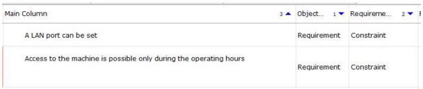
ReqEdit multi column sorting displayed by numbered arrows in the column headers
